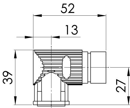
Rotary angle socket - mating connector
