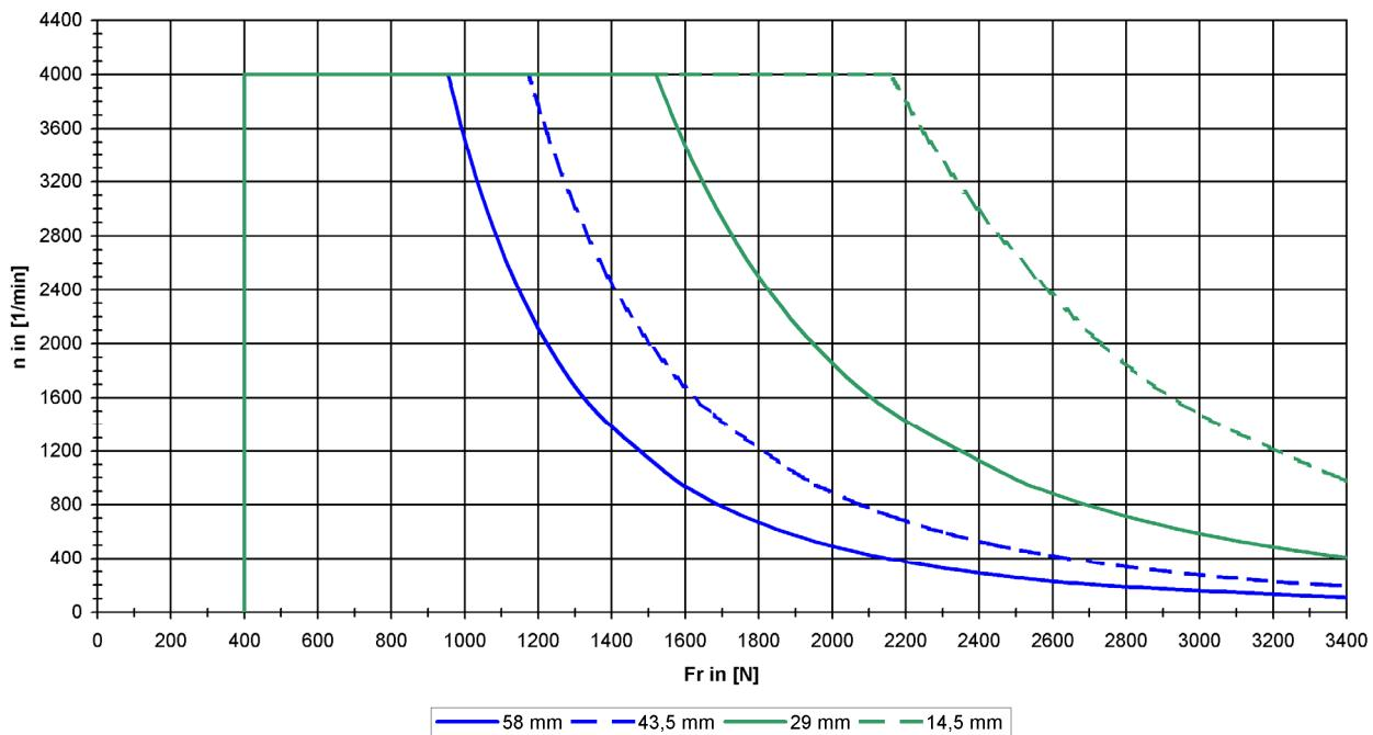
Note: 20,000 grease consumption duration at  $n_{\text{effective}} \leq 1,150$  rpm
