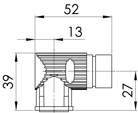
Speed-Tec - rotary angle socket
