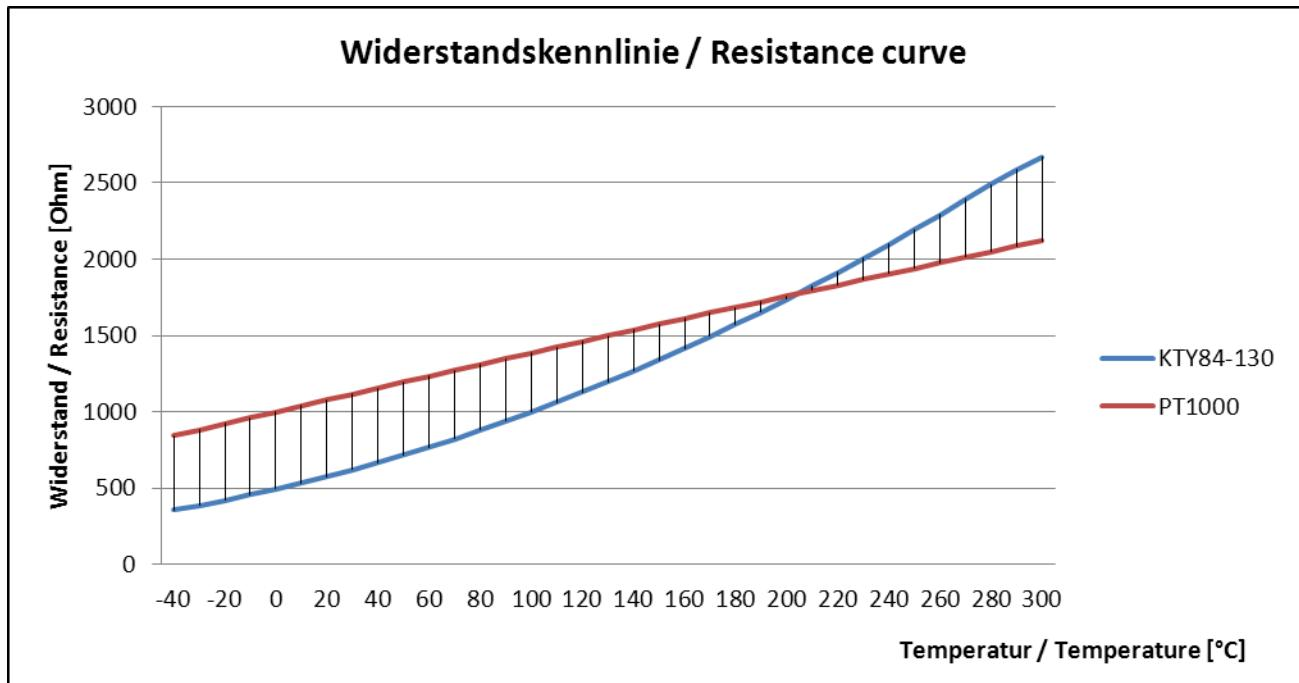
The motor temperature is continuously monitored using temperature sensor type KTY84-130,
