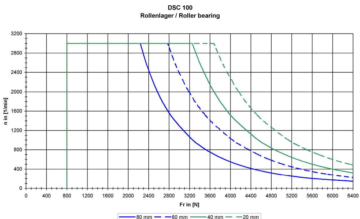
Note: 20,000 grease consumption duration at  $n_{\text{effective}} \leq 850$  rpm
