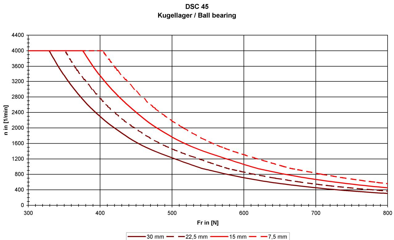
Note: 20,000h grease consumption duration at  $n_{\text{effective}} \leq 4,000$  rpm
