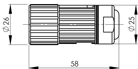
Rotary angle socket for ECN1325/EQN1337 encoder (mating plug cannot be supplied separately)
