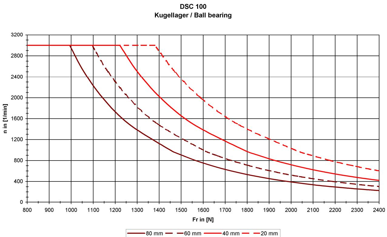
Note: 20,000h grease consumption duration at  $n_{\text{effective}} \leq 3,000$  rpm
