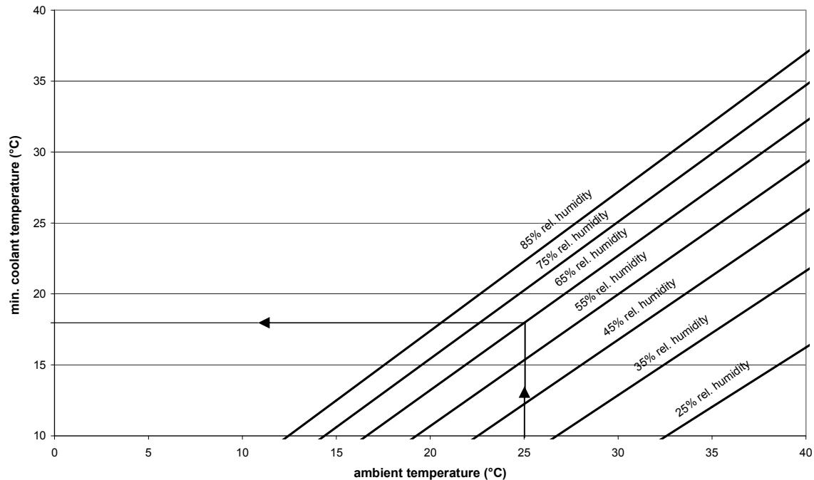
The allowed coolant temperature depends on relative humidity and ambient temperature. For example with an ambient temperature of 25 °C and a relative humidity of 65% the minimum coolant temperature is 18 °C. Because these are limiting values on practical side a coolant temperature greater than 18 °C should be used. If this minimum coolant temperature will be under run the two-point controller of Baumüller drive must be used to avoid condensation.
