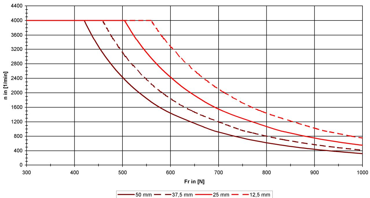
Note: 20,000h grease consumption duration at  $n_{\text{effective}} \leq 4,000$  rpm
